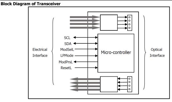
The QSFP AOC has miniature optical engines embedded into each end of the cable assembly. The engines interconnect 4 independent transmit/receive lanes.
